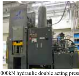
3000kN hydraulic double acting press (by AMINO Co.) Max. ram speed : 50 mm/s
